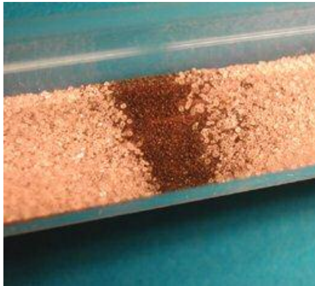
FIG. 13. Bands in white table salt and fine, black sand that spontaneously formed when the cylinder was continuously rotated around its axis. 16
