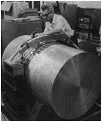
Figure 2: This is a picture of Weber with one of his resonant mass detectors. A passing gravity wave would cause the bar to vibrate, which would then be detected by the piezo-electric chips along the waist of the bar. [Hans C. Ohanian, Remo Ruffini, Gravitation and Spacetime 2 nd ed. (W. W. Norton and Company, New York, New York, 1994) p. 281]
